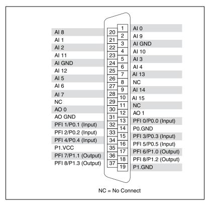
Figure A-1. NI 6232 Pinout
